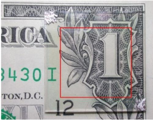
Photograph of a 1 inch by 1 inch glass substrate patterned with spin-coated zinc oxide transparent transistors, sitting on the top of a dollar bill. There are 56 transistors in the red box.
