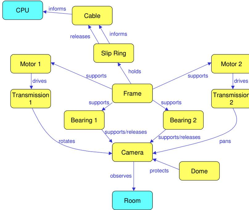
Figure 2: Simplified FAA Model for the Camera System
