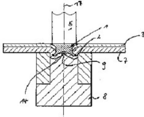
The idea of a self-piercing rivet is not, of course, a totally new idea. From the perspective of ideality, the concept of a rivet that doesn't require the prior need to drill a hole is very attractive. It means production time saving, tool wear reduction, less waste material production and last but not least, an often significantly stronger join.
