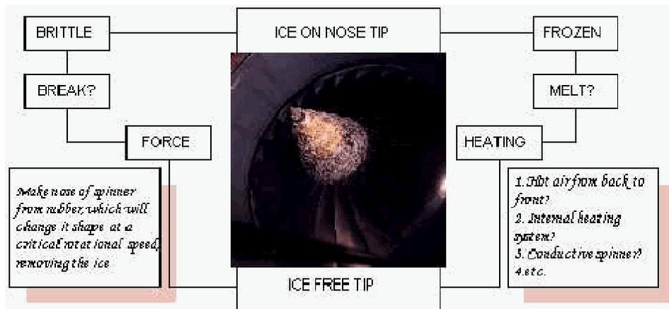
*Figure 2: Gas-Turbine Spinner Problem Solution Routes*
