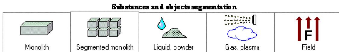
**Figure 3: 'Substance and Object Segmentation' Trend**
