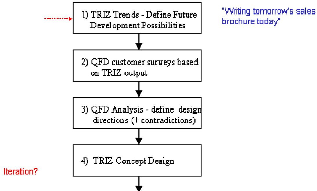
Figure 7: Defining The Customer Needs Using QFD and TRIZ
