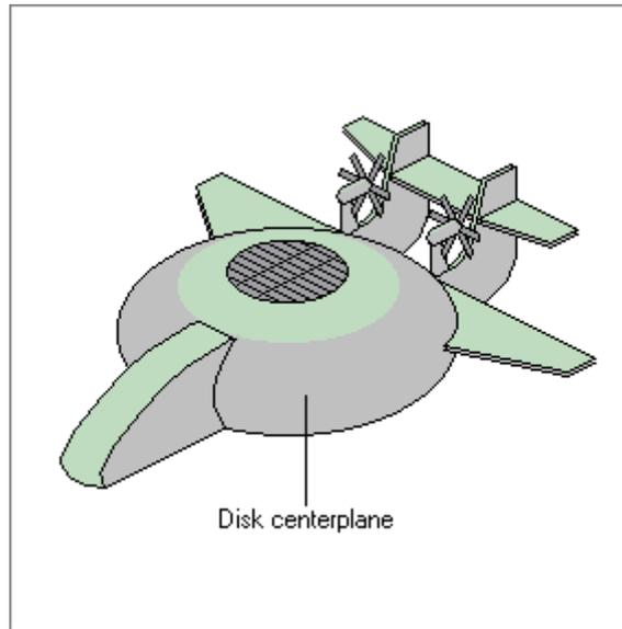
Figure 2: 'Aerostatic Aeroplane' - Russian patent 1,550,790
