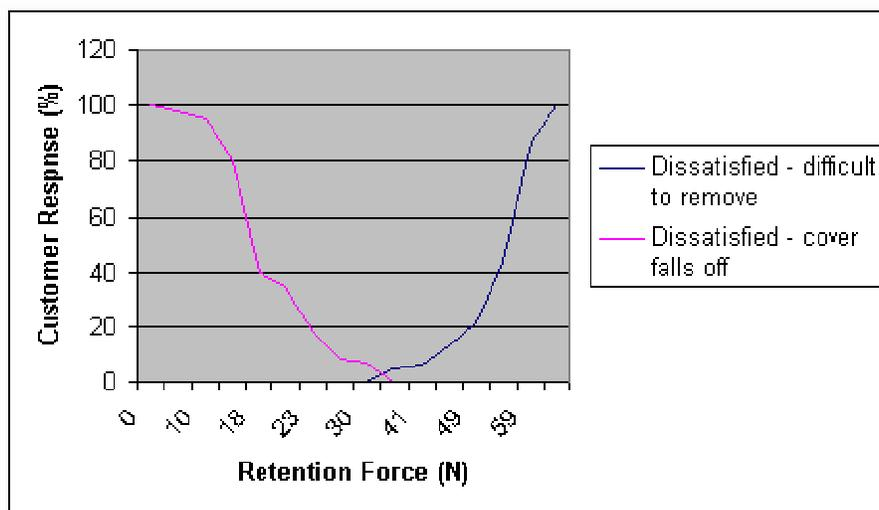
Figure 5: Wheel Cover Retention Force Design Point Selection
