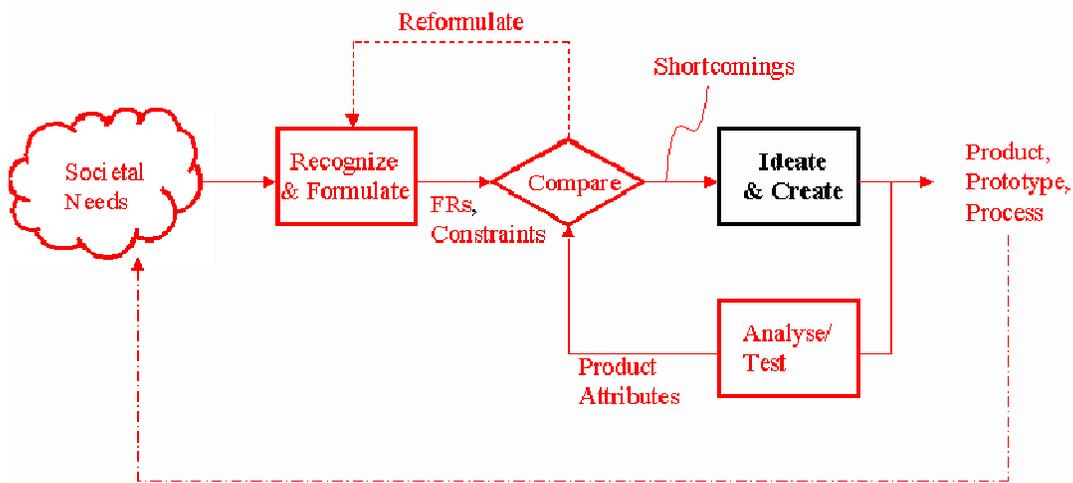
Figure 1: Schematic of Design Process (based on (1), Fig 3.10)
