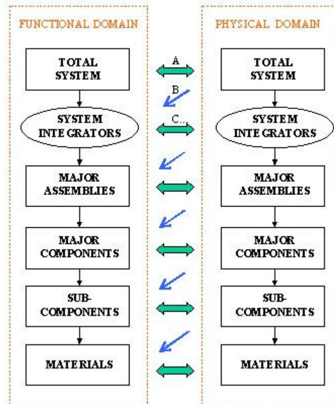
Figure 7: Hierarchical Nature of Functional Domain – Physical Domain Mapping
