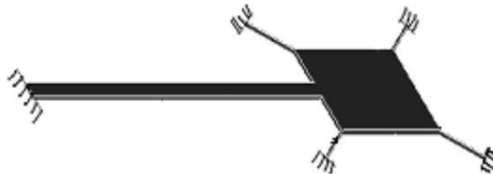
Fig 2b. Polysilicon cantilever mirror with supports
