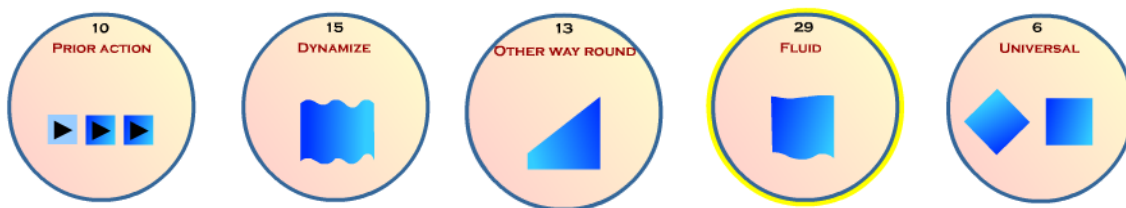
Figure 8: Inventive Strategies Most Likely to Resolve JIT versus Risk Conflicts (based on Reference 11)
